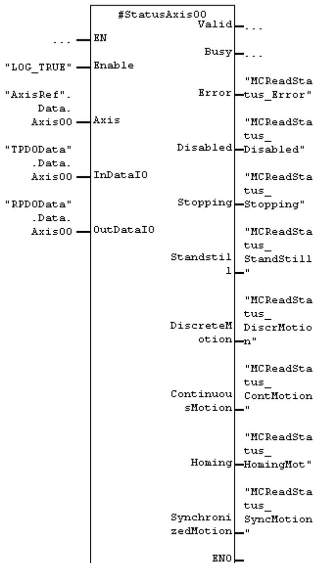
In the STAT-area of a Container-FB instantiated MC\_ReadStatus\_C3 with the instance name StatusAxis00.
