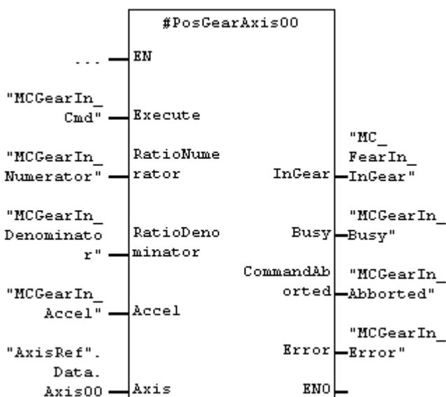
In the STAT-area instanciated MC\_GearIn\_C3 with the instance name PosGearAxis00.
