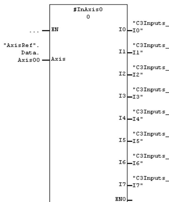
In the STAT-area instanciated C3\_Input with the instance name InAxis00.
