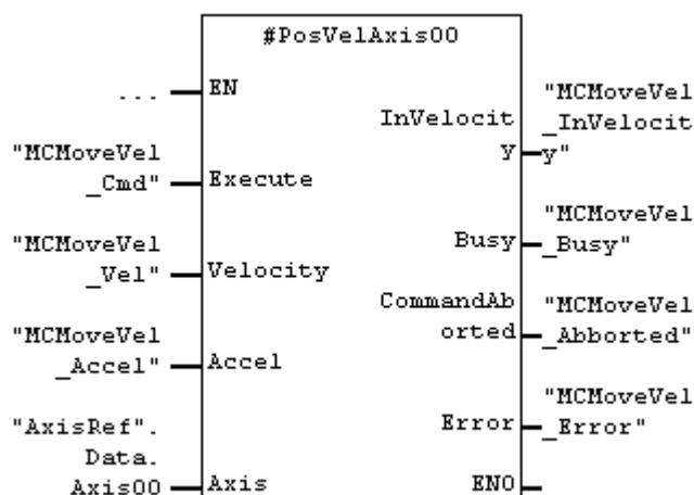
In the STAT-area instantiated MC\_MoveVelocity\_C3 with the instance name PosVelAxis00.
