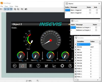
Automatical simulation: Starts the SimuStage together with the Siemenssoftware S7-PLCSIM (what must be installed at the same PC). The process data come from S7-PLCSIM (not from PLCSIM Advanced – this is for 1200/1500CPUs). Of course, S7-PLCSIM does not simulate INSEVIS-SFCs/SFBs.
